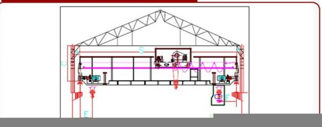
l established manufacturer and exporter of EOT cranes with double girders, that find application for the purpose of lifting & r 10 T and for span of more than 30 m. Comprising of 2 torsion-free box girders, these EOT cranes such as double girder eo cranes, material handling eot cranes etc., are compatible, when heavy loads and wide spans are required. These double girde fered by us in the load capacities of up to 100 T and with spans up to 50 M.
